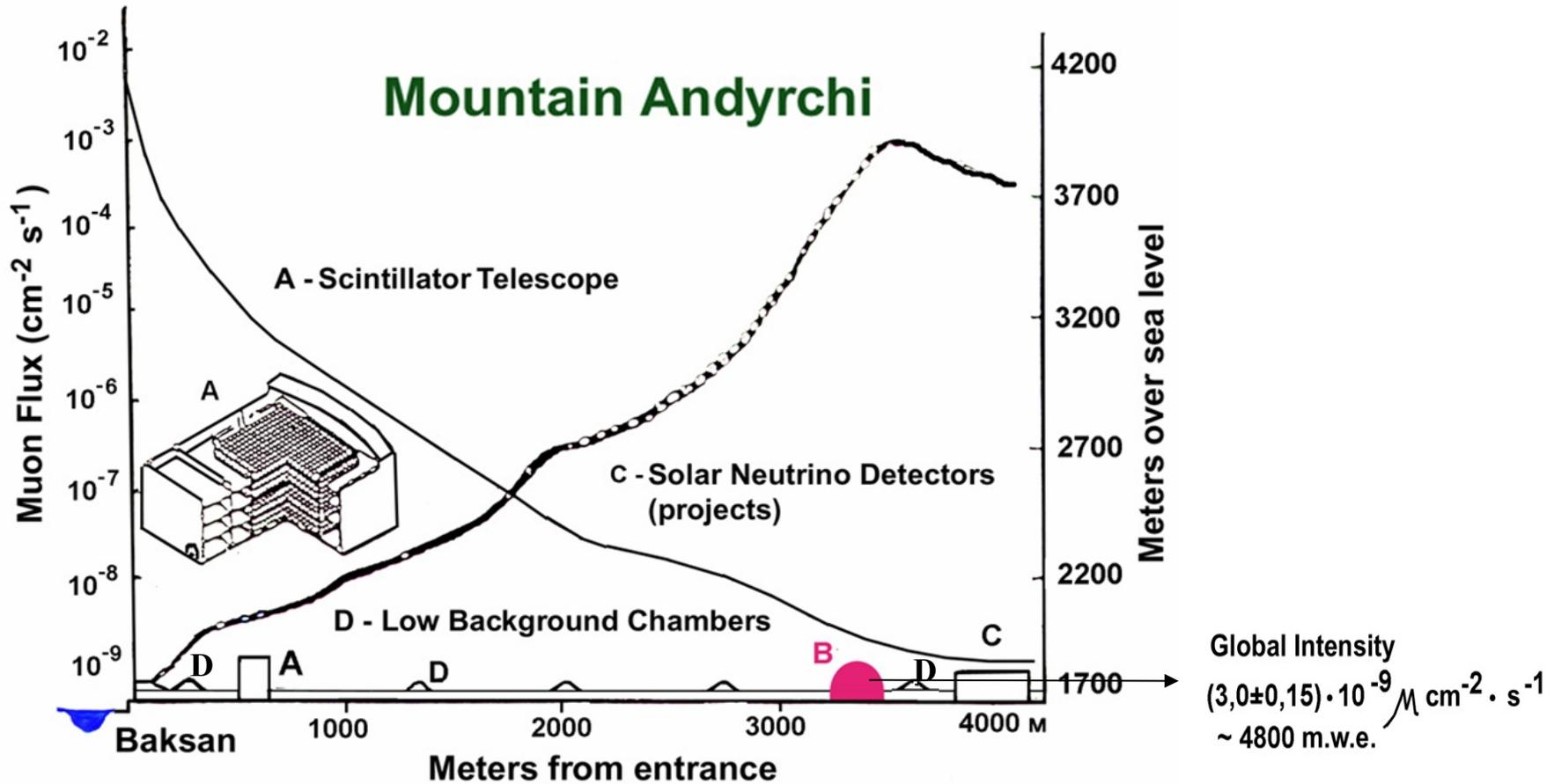
*Schematic view of a section of the Andyrchy slope along the adit (right scale) and dependence of underground muon flux on the laboratory location depth (left scale).*
